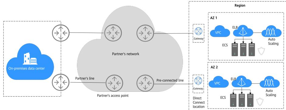
Connections support redundant configuration. If there are two connections terminated at different locations in the same region, they can work in an active/standby pair to back each other up. If one connection becomes faulty, the other will take over, ensuring stable services.
